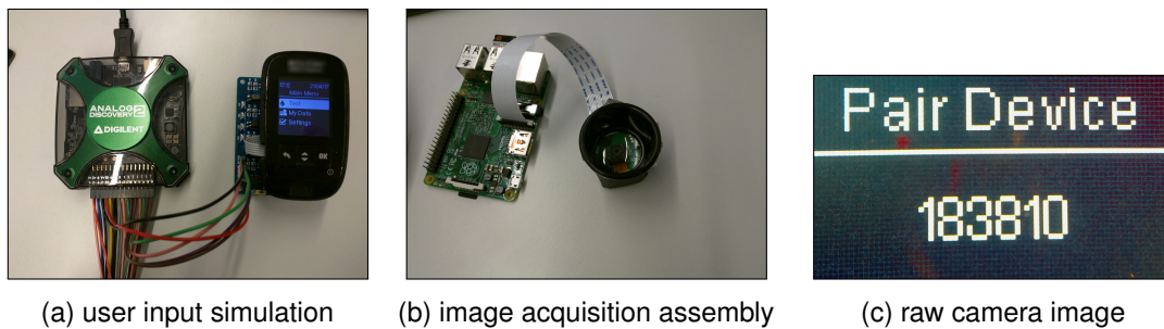
Figure 8.2: Setup for automated passkey acquisition
